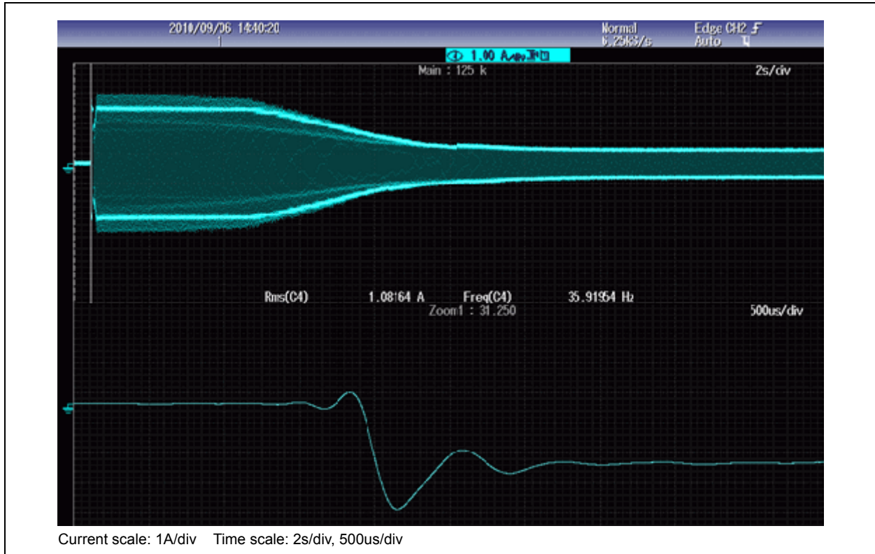
FIGURE 34: CURRENT FOR COLD LAMP; ZOOM OF THE TAKE-CURRENT
