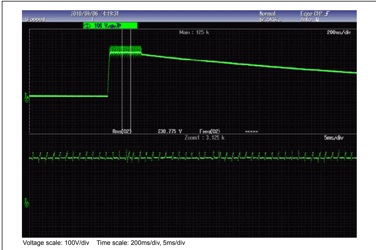
FIGURE 30: OPEN VOLTAGE WAVEFORM AND IGNITION FAILED PROTECTION
