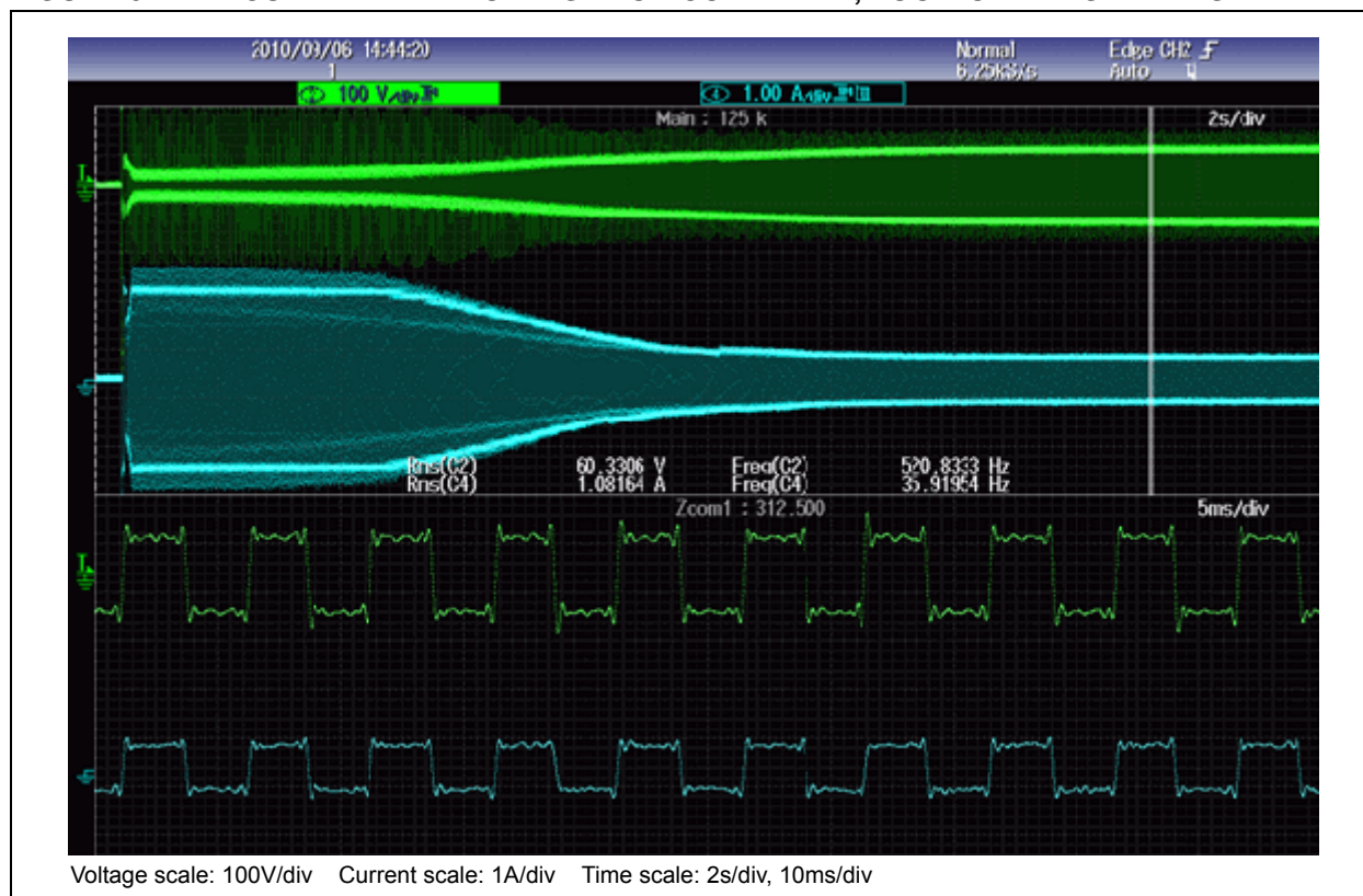
FIGURE 37: CURRENT AND VOLTAGE FOR COLD LAMP; ZOOM OF THE STEADY STATE
