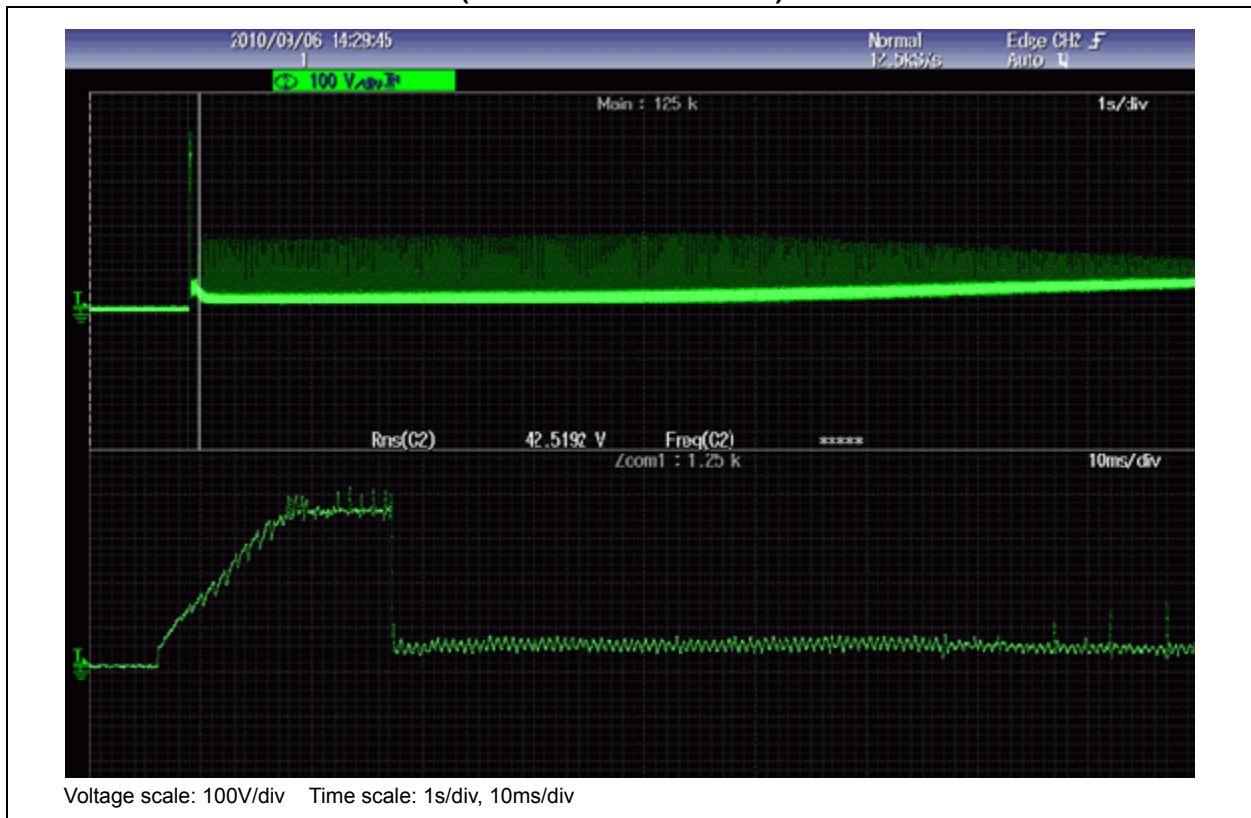
FIGURE 31: DC BUS VOLTAGE (SUCCESSFUL IGNITION) OF BREAKOVER POINT
