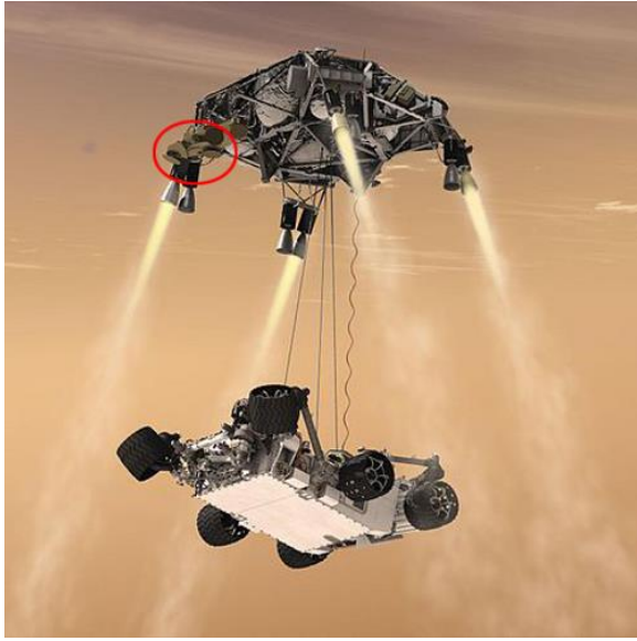
JPL Mars Curiosity Sky Crane and Rover with location of Wenzel Frequency Synthesizer circled in red.
