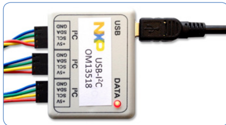
OM13518 Universal USB to I 2 C-bus RTC interface dongle
